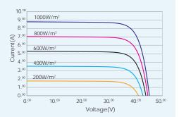
Average efficiency reduction of 4.5% at 200W/m<sup>2</sup> according to EN 60904-1.
