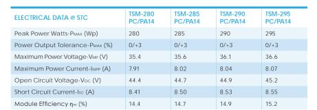
Values at Standard Test Conditions STC (Air Mass AM1.5, Irradiance 1000W/m², Cell Temperature 25°C).
