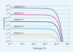
Average efficiency reduction of 4.5% at 200W/m<sup>2</sup> according to EN 60904-1
