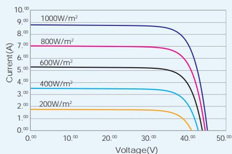
Average efficiency reduction of 4.5% at 200W/m<sup>2</sup> according to EN 60904-1.
